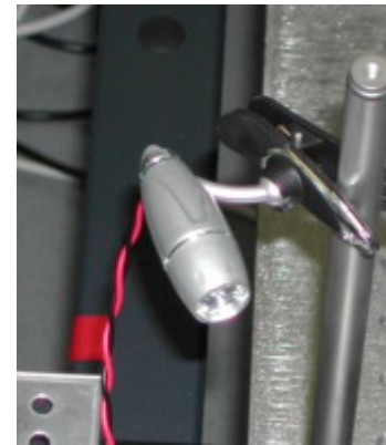
IR gating 848nm 23mW LED
